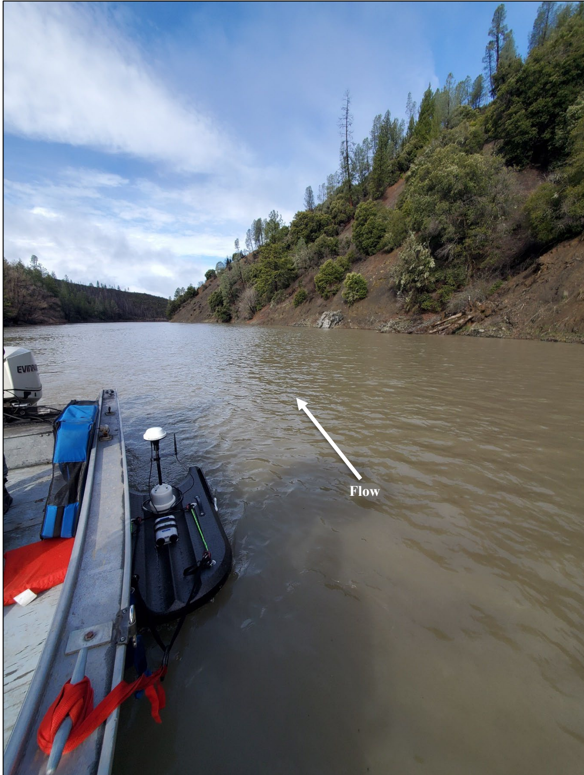
Photograph 7. On January 22, 2024, US Fish and Wildlife Service provided jet boat assistance to collect a high flow measurement using an ADCP mounted to a riverboard. Measured discharge was 2,740 cfs, later adjusted by drainage area to 2,660 cfs. This measurement was taken at approximately 1.7 miles downstream from the gage site.
