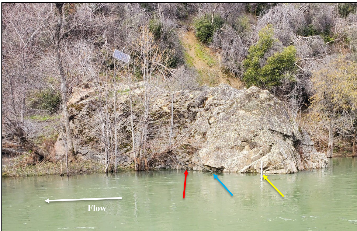
Photograph 3. Gage pool showing staff plate (yellow arrow), DTS-12 turbidity/temperature sensor (blue arrow) and primary and backup pressure transducers (red arrow). The gage solar panel can be seen above the rock outcropping. Photo taken on January 30, 2024, and flow was measured at 488 cfs.
